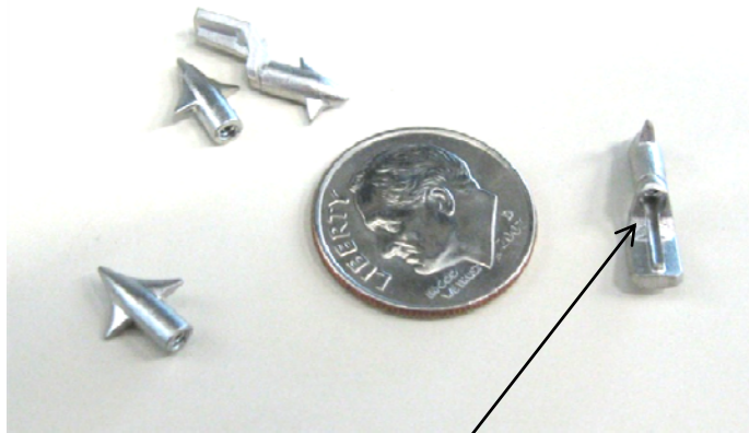
Four cavity tool 0-80 auto-unscrewing thread
